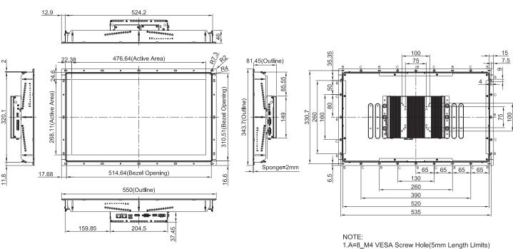
1.A=8\_M4 VESA Screw Hole(5mm Length Limits) 2.B=16\_9\*4 Oblong Hole3.C=8\_4.D=12\_M5 Screw 3.C=12\_M4 Screw Hole
